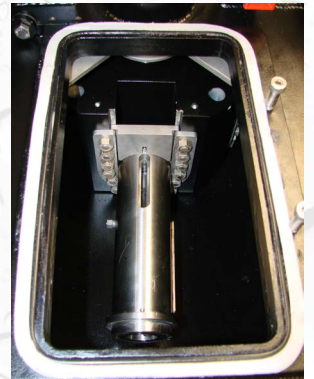
A Test Cell Attached to the Rotor
