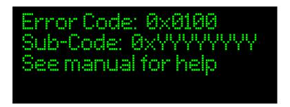
Error 0x0100 indicates a self-test failure and 0xYYYYYYYY is a code specific to the type of error detected. If the self test fails, first cycle the power. If the error remains, change the batteries and/or switch to an alternate power source. If the error still remains, the meter will need to be repaired by a qualified technician.
