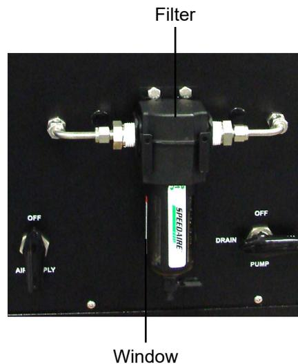
14. Turn the Air Supply valve ON.
