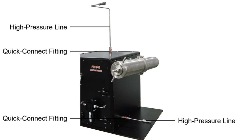
8. The port on the bottom cell cap should already be turned to the correct angle to line up with the high-pressure line. However, on the top cap, the port may need to be rotated to line up with the high-pressure line. If so, use an adjustable wrench to turn the inner portion of the cap so that the port is at the correct angle to line up with the high-pressure line.
