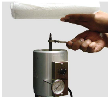
Safe Release of Pressure from a Cell
